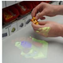
A 3D model showing the assembly instruction is projected onto the manual workstation and guides the user step by step through the assembly process.
