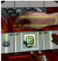
Support for the assembler: At the manual workstation the mobile projection shows the user where to grab which part.
