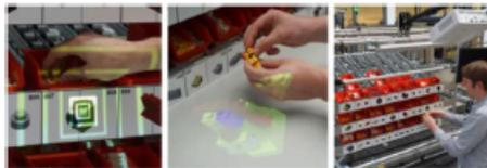
Support for the operator. An interactive application that displays and highlights the location of the part to be assembled.
