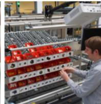
The projection-based AR environment is tested in the virtual assembly system of the SmartFactoryOWL. Source: CST
